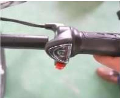
Slide the Twist throttle into the right side of the handlebar and get a feel of twisting the throttle.
