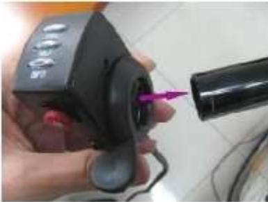
Slide the thumb throttle into either side of the handlebar that you feel comfortable with.
