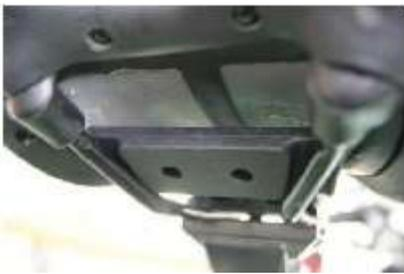
Slip the mounting plate under the saddle support
