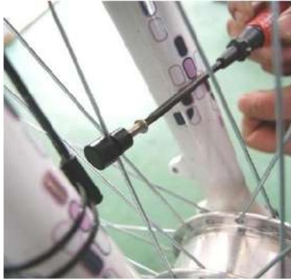
Mount the magnet to the spokes using a Philips screwdriver
