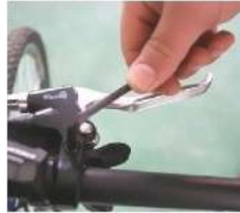
Then tighten using a 5.0mm Allen Wrench
