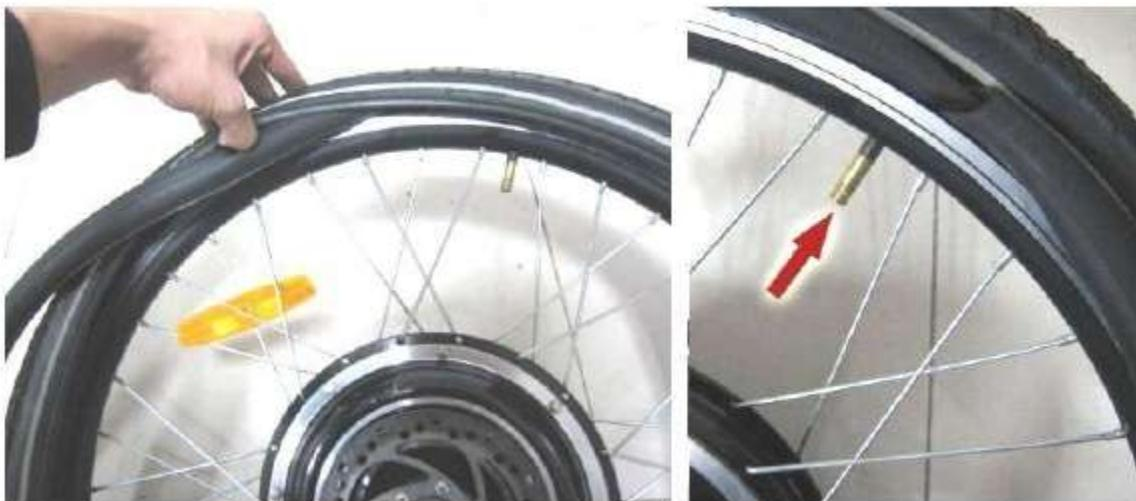
Place the rest of the tube between the rim and the tire and pull the tire over the rim. Then pump it up, check for leaks and you're done assembling the wheel.
