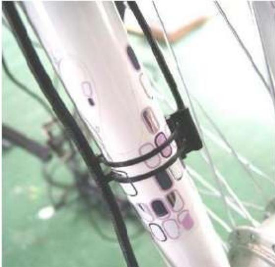
Mount the sensor to the fork using the rubber bands
