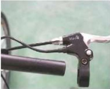
Slide the hand brakes into both sides of the handlebar. Find a comfortable position.
