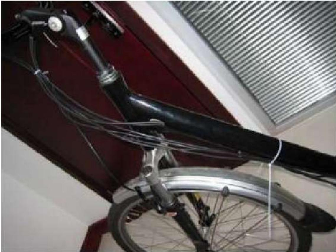
Note: As a suggestion, after you tied your cables, rotate your handlebars to see if the movement is smooth and undisturbed.
