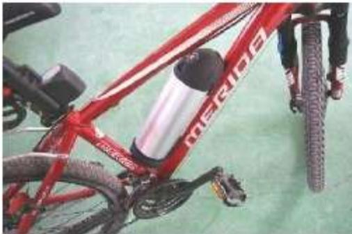
Put the battery into the case. And connect the battery to the controller
