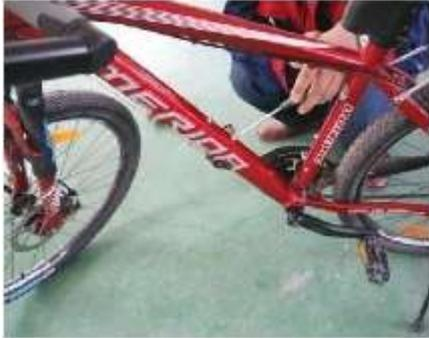
Remove screws for bottle holder from frame
