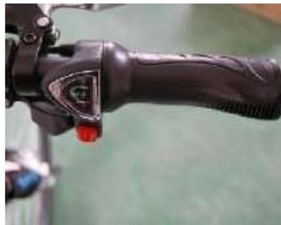
When you feel comfortable with the position, use the 3.0mm Allen Wrench and secure it into place.
