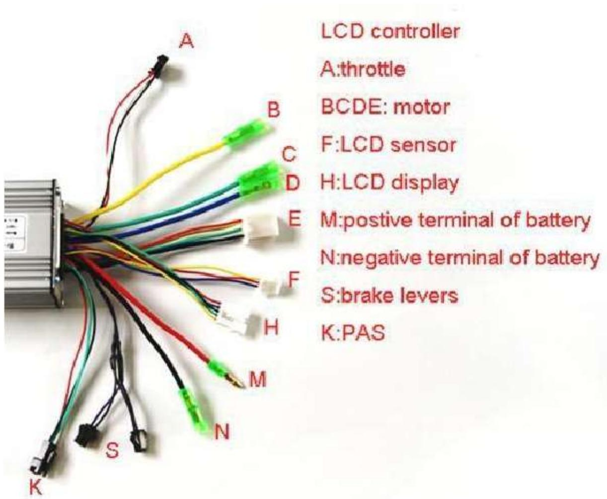
LCD meter: it has two parts, one is the LCD display, the other is LCD speed sensor. LED meter : everything is same to LCD ,just don't care about speed sensor connector
