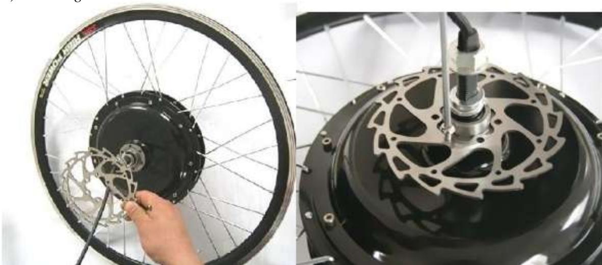
Note: Please check your disc brake diameter. In most cases, 140mm disc brake are used for the rear wheel while 160mm are used for the front wheel.
